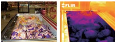
Frozen Chicken – This thermograph shows frozen chickens in a grocer's freezer. By scanning frozen goods in the freezer unit, problems such as improper temperature can be avoided or quickly remedied and food spoilage or foodborne illness can be avoided.
