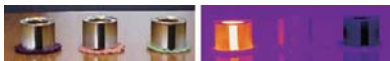
Graph 2.6 Three aluminum cans with partially oxidized surfaces and a strip of black electrical tape. The can on the left is hot, middle can is ambient and right can is cold.
